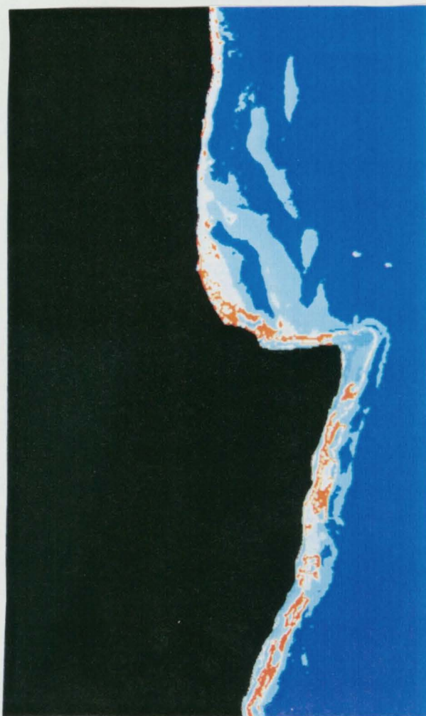
Figure 7.2. An unsupervised classification of the Island View image using principle components 2, 3 and 4 created with bands 1, 2, 3, 6 and 8. Areas of red are Monostroma spp. and the boxed area indicates where the accuracy assessment was performed.
