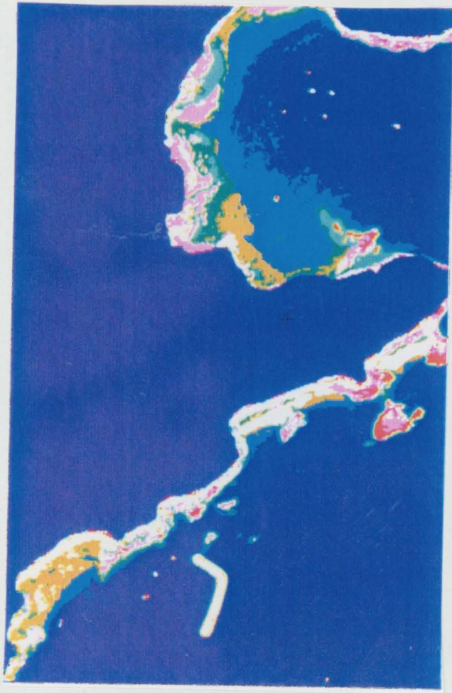
Figure 7.1. An unsupervised classification of the Sidney image using principle components two, three and four from a PCA created with bands 1, 2, 3, 6 and 8. Areas of red are Fucus distichus , green are Enteromorpha spp. and/or mixed Chlorophytes, purple areas are beds of the Chlorophyte Blidingia spp. Green areas along the waterline of Sidney Shore are areas of the Chlorophyte Monostroma spp. Brown areas are organic rich muds with sparse areas of Chlorophytes covering them. Boxes A and B are areas where an accuracy assessment was performed.
