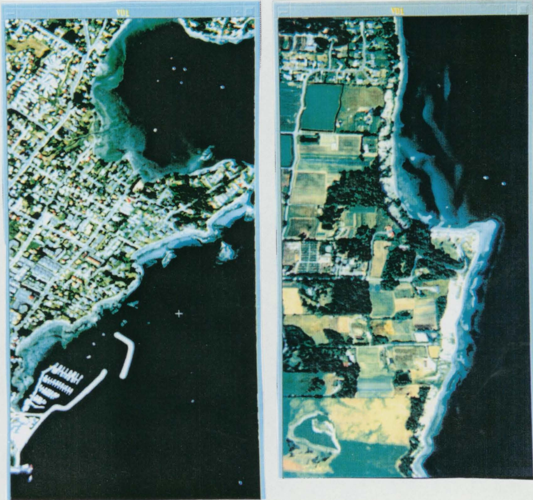
Figures 5.2 and 5.3. Near true colour composites using bands 6, 3 and 1 for Roberts Bay, Sidney Shore and Island View Beach. Image size is 512 lines by 512 pixels, but has been stretched to 1024 lines to reflect the 2:1 aspect ratio of the pixels at the altitude at which the data were acquired.
