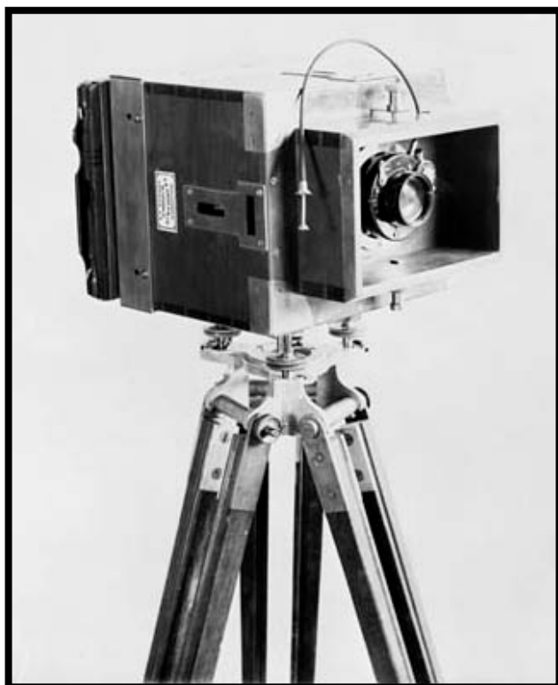
Figure 8: A photograph of one of the cameras used for the topographical survey of Canada. Source: L&AC Mkan m. 3389791
