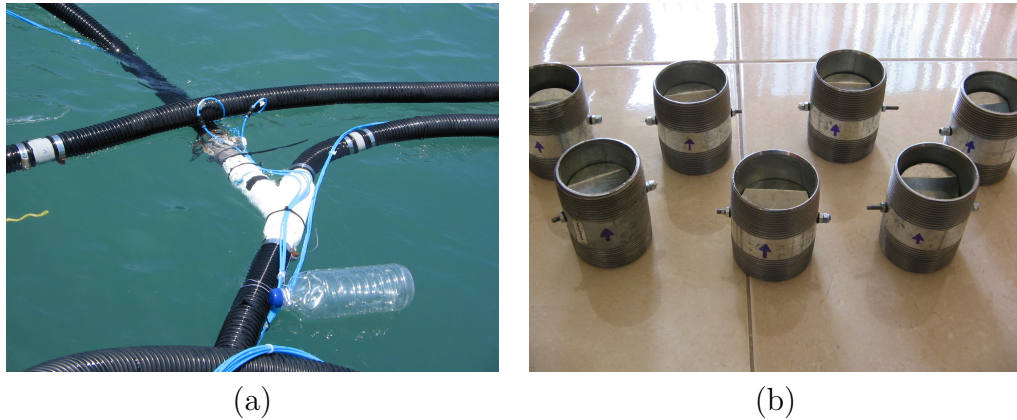
Figure 5.4: (a) Actual conduits assembly with floaters; (b) check valves.
