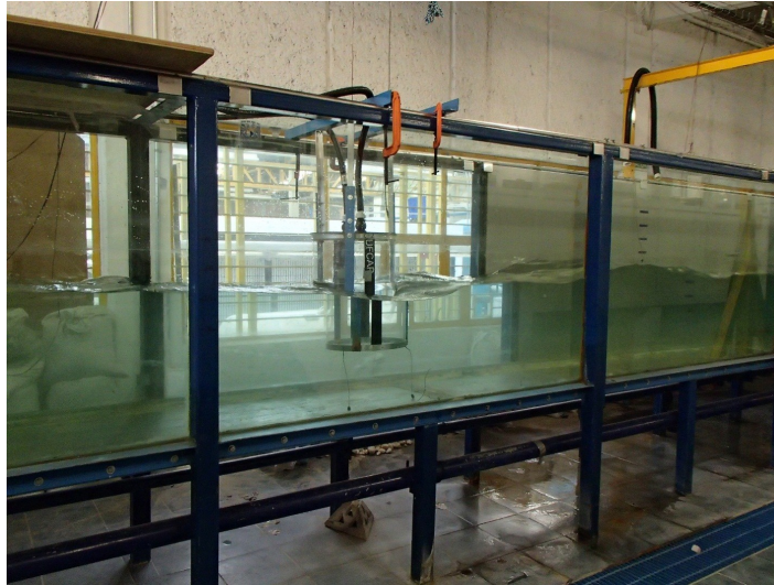
Figure 6.6: Single air-chamber test in wave flume.
