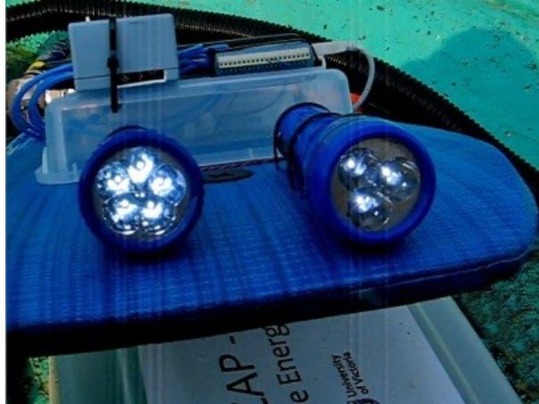
Figure 5.14: Eight LEDs lighted by the UFCAP WEC. Control-board over the boat.
