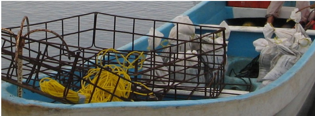
Figure C.2: Mooring metal basket and sand weights.
