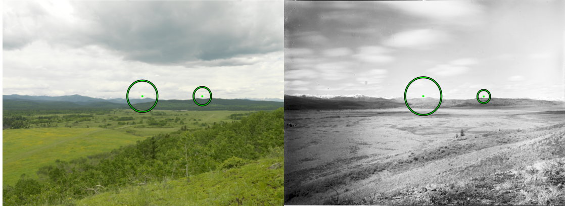
Figure 32 An image pair in our dataset where few correct matches were found. Notice that the majority of the landscape has changed, leaving very few stable features to be detected and matched. The circles represent the scale of the local features. In this case (DoG/SIFT, distance threshold = 250), 334 false matches existed in the proposed match set (not shown).
