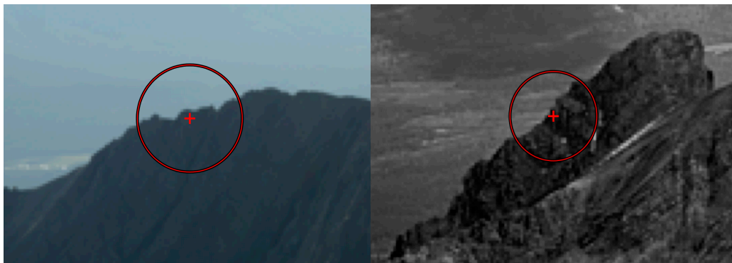
Figure 33 A false match that occurred because of the rotation invariance of the descriptor.
