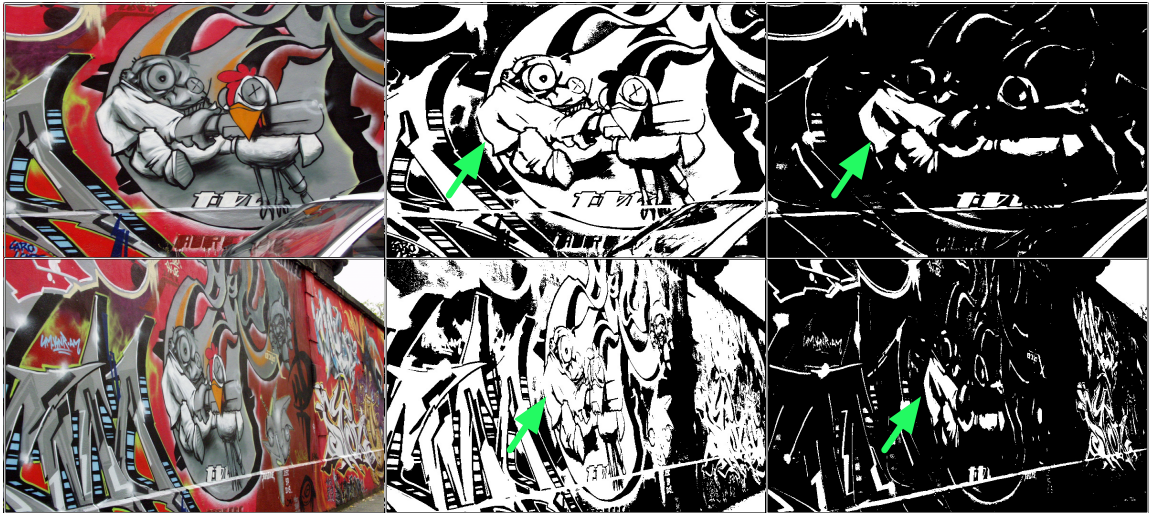
Figure 13 The image above shows two images of the same scene that differ on viewpoint change. The black and white images in the rows adjacent to these images show two binary threshold images. The thresholds used are 100 and 150. The green arrows demonstrate an example of a connected component that is stable over an intensity change of the surrounding area. Note that the feature is consistent over viewpoint change.
