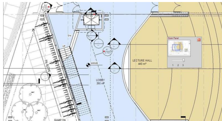
Figure 9. Screenshot displaying a zoom panel and a Tile displayed a magnified sheet bounded by a blue rectangular box on the zoom window.
