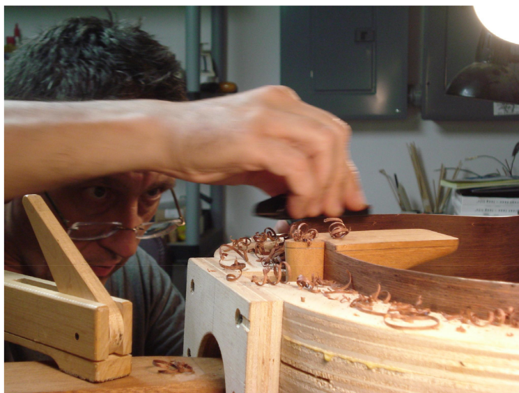
FIGURE 2 Sasha scraping the sides of a guitar-in-progress, aided by a metal plane and guided by his sight, touch, and intuition.
