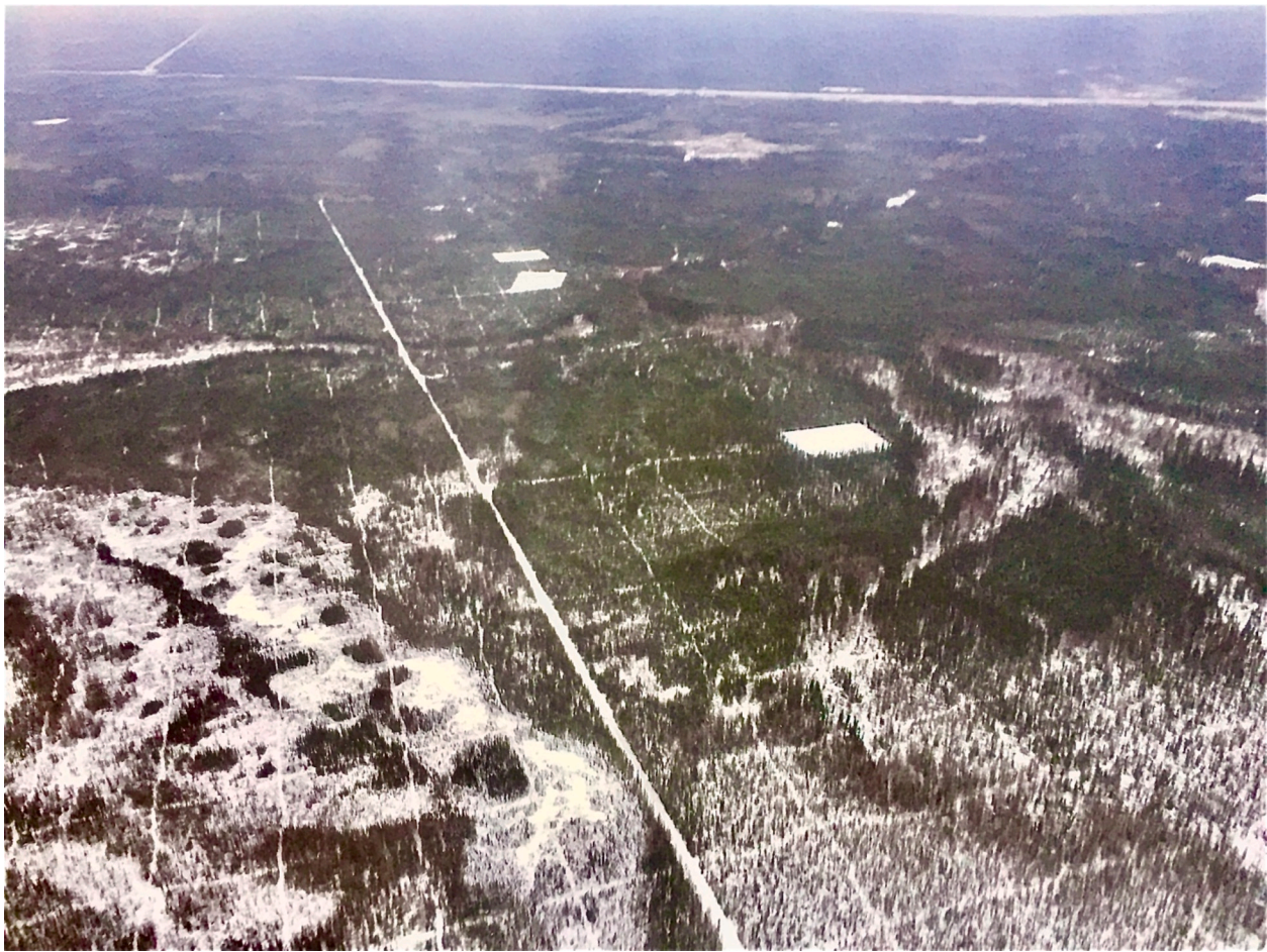
Fig. 2. Anthropogenic features include linear features such as roads, pipelines, seismic lines, and 3-D seismic lines (“hashtag” patterned), and block (polygonal) features such as cutblocks (irregular shapes) and well sites (small square shapes).
