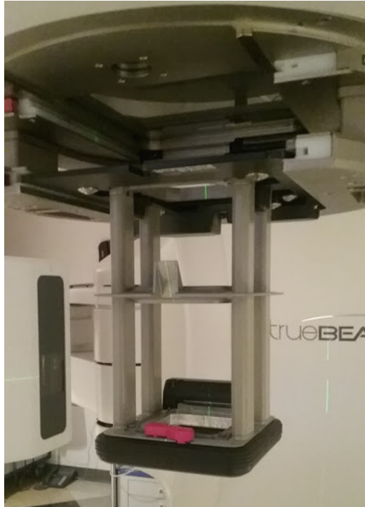
Figure 2.10: Photo of a 10 \times 10 \text{ cm}^2 electron applicator and cone mounted on the TrueBeam.
