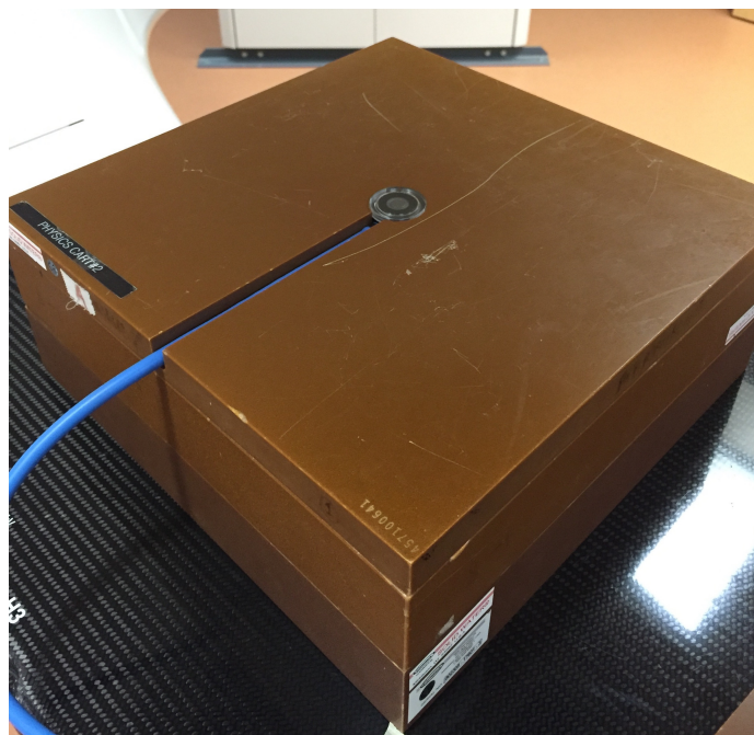
Figure 3.1: Markus ionization chamber in Solid Water for output measurements. Various thicknesses of Solid Water were stacked on top of this set up prior to measurement. Photo credit: Evan Maynard.
