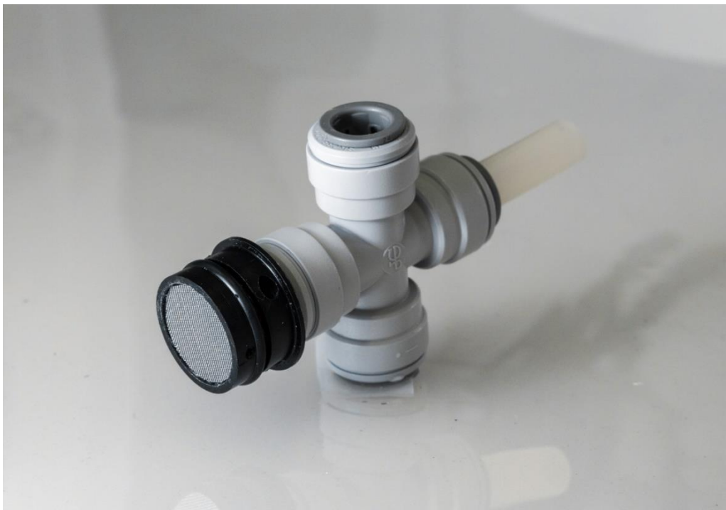
Figure 0-4 End connector of the regenerator consists of one push-to-connect tee, a mesh screen and an o ring.
