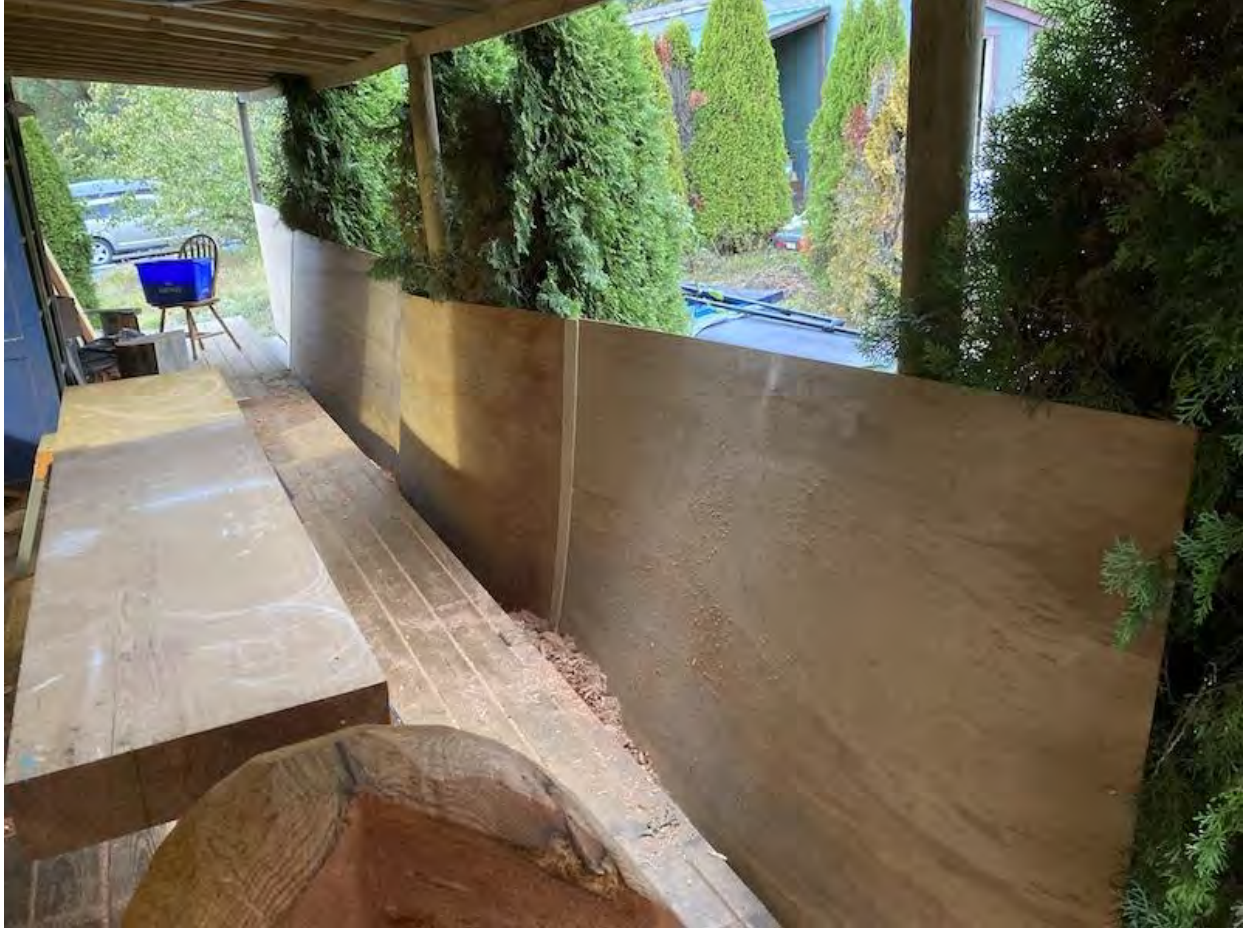
Fig. 17. Four sheets of \frac{1}{8} " plywood joined together to form the inside wall of the Untitled TETÁCES map, which is almost ten metres in length. 228
