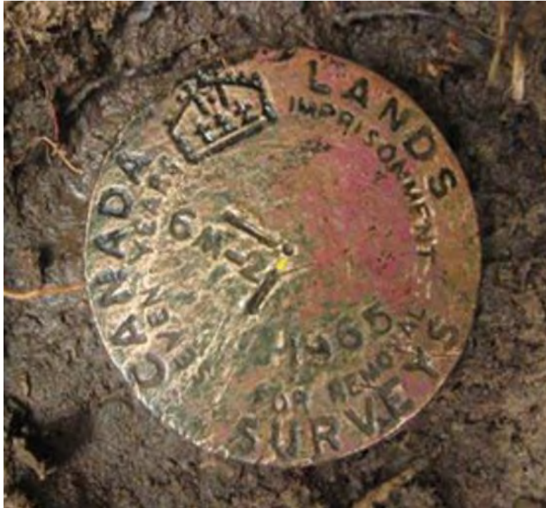
Fig. 2. An example of a surveyor's "monument" or marker. Note the following warning: "SEVEN YEARS IMPRISONMENT FOR REMOVAL." 42
