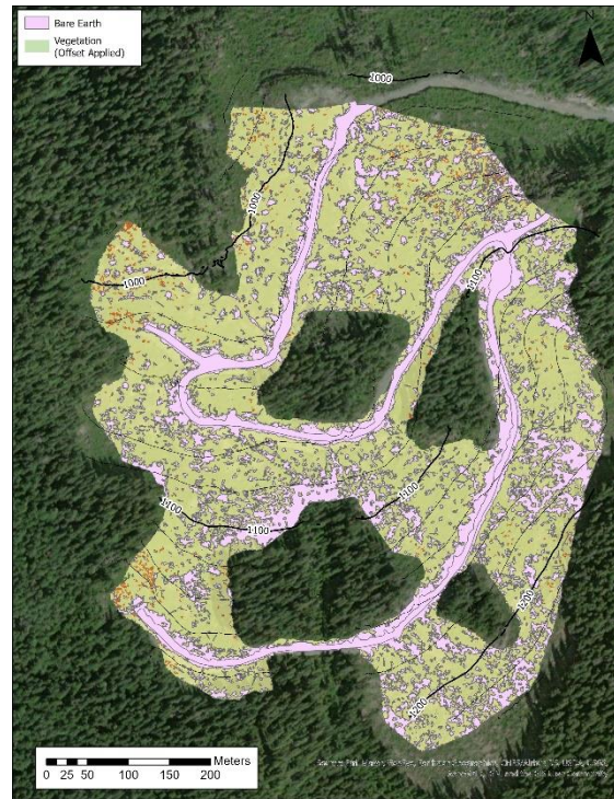
Figure 18. The study plot divided into vegetated and non-vegetated areas by a supervised classification process. Areas classified as vegetated have offsets applied to them.
