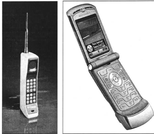
Figure 3.5: The mobile telephone has been the subject of exceptional advancement over the past twenty years. The first cellular telephone, Motorola's DynaTAC 8000X (L), weighed 795 grams and lasted 30 minutes per charge. That was 1984. Motorola's latest mobile, the RAZR V3 (R), tips the scales at a svelte 95 grams and yields up to seven hours of talk time. (Images are not to scale.)
