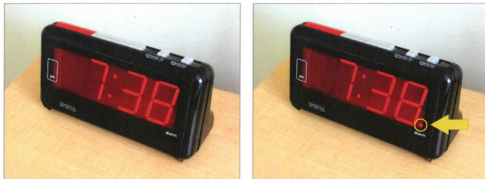
Figure 3.7.1b: Digital alarm clocks commonly use a single indicator to differentiate between the interface modes for (L) time setting and (R) alarm setting.
