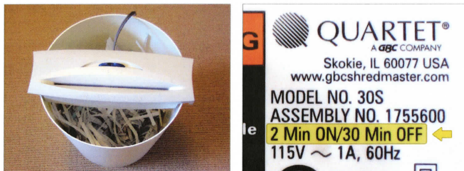
Figure 3.7.3: Electric motors in light-duty appliances, such as hand blenders, hair dryers, and electric drills, and are not designed for continuous operation and typically require a period of rest after prolonged use. For this (L) paper shredder, a 30-minute cool down period is required after two minutes of continuous operation (R). Users unaware of this behaviour may think that the shredder has malfunctioned.
