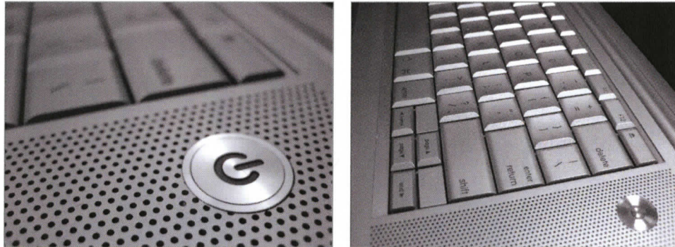
Figure 2.2.2: The power switch on this Apple PowerBook has been given greater visibility by placing it apart from the other buttons and keys. On some Macintosh models, the power light is also backlit for identification in darkened environments.
