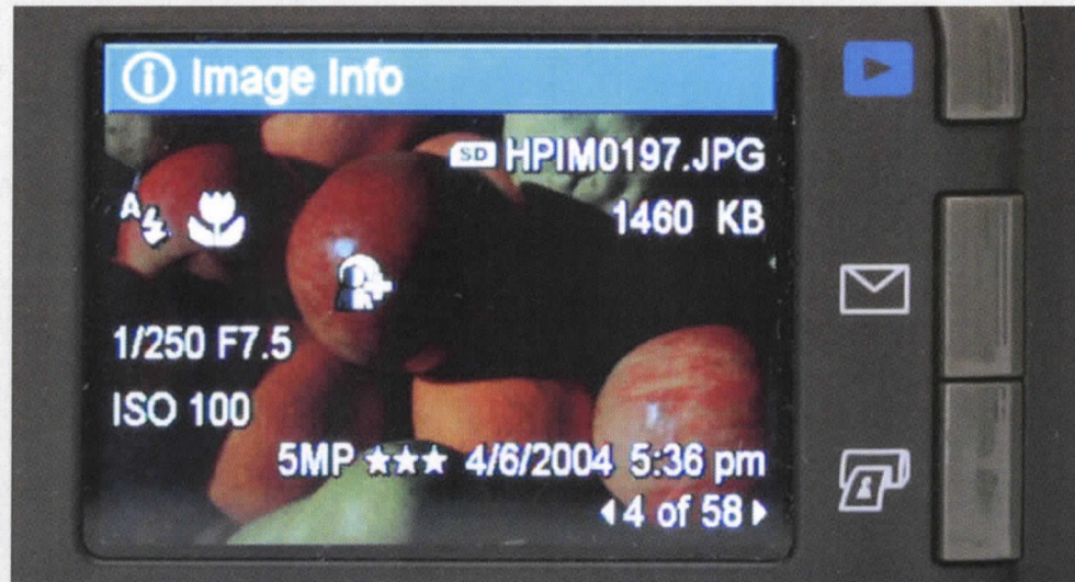
Figure A4: The HP PhotoSmart R707 uses a colour-coded title bar and icon to announce the current operating mode to the user. No colour or icon is used more than once.
