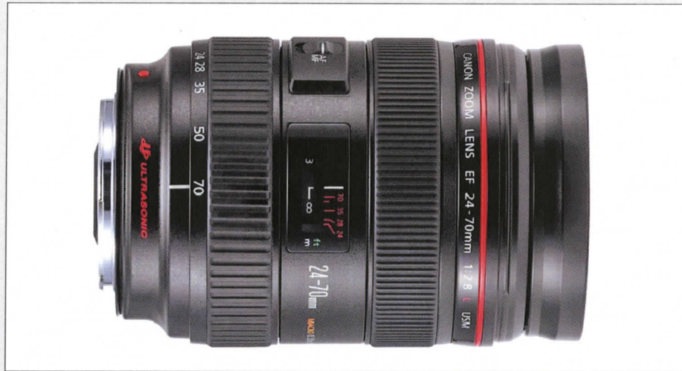
Figure D4: The zoom and focusing rings on the Canon EF 24-70mm f/2.8 L USM lens operate in similar manners: for a distant object, turn the zoom ring counter-clockwise to zoom in and turn the focus ring counter-clockwise to focus. In photographer's parlance: turning the zoom ring counter-clockwise increases the lens' focal length; turning the focus ring counter-clockwise moves the focal point towards infinity. In both cases, the "numbers" for both parameters become larger with a counter-clockwise turn.
