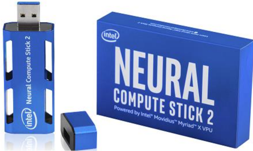
Figure 4: The Intel Movidius NCS2 used for computation [37].
