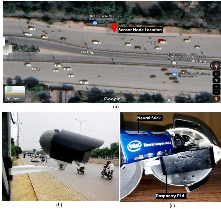
Figure 10: The sensor node installation: (a) overhead location, (b) field view, and (c) inner view.
