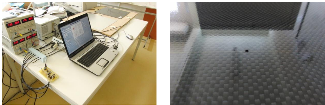
Fig. 5.37: Composite experimental setup and simulated damage
