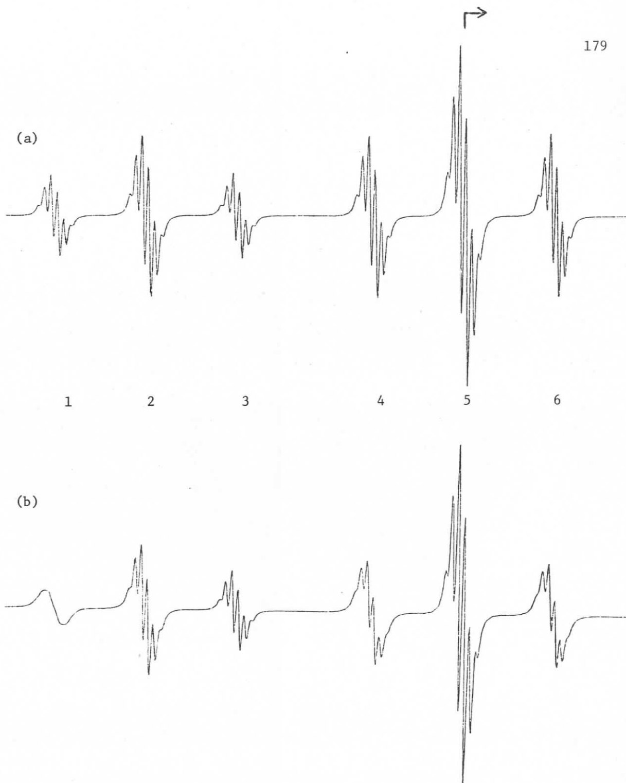
FIGURE 61: Simulated low temperature exchange spectrum of 1-hydroxycyclohexyl radical (81), (a) at fast exchange (ca. -70°C), (b) at slower exchange (ca. -90°C). (Second order splittings not included.)
