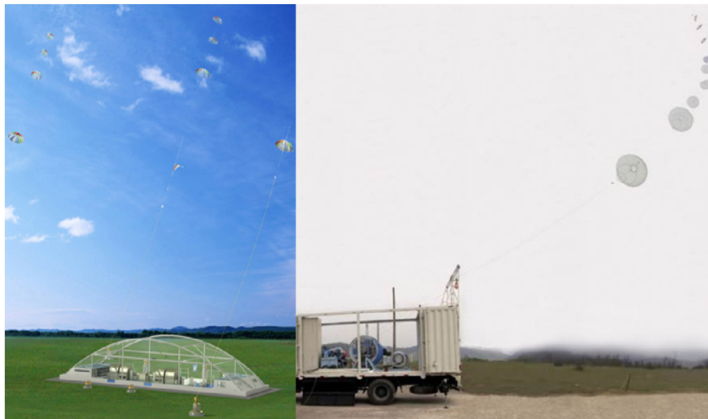
Figure 1.7: An artistic vision (left) and an implemented prototype (right) of an umbrella-ladder system [6].
