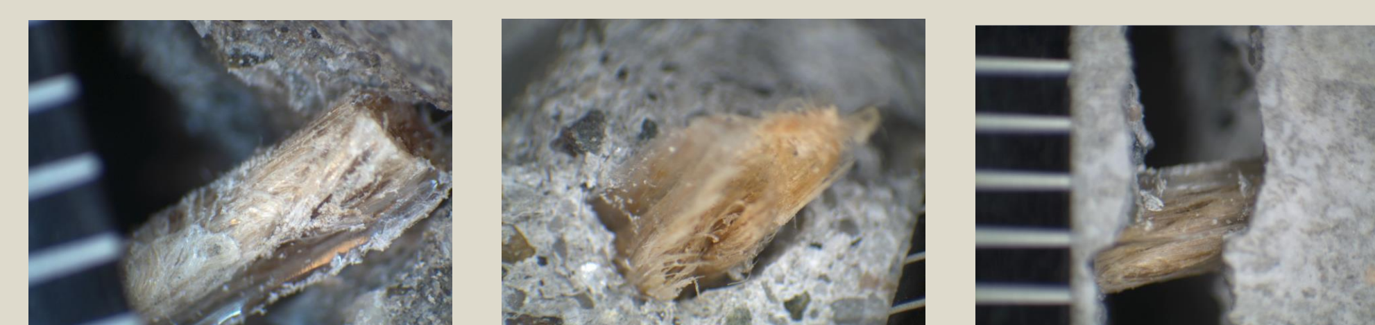
Figure 7: From left: unaged twine, broken aged twine, aged twine (Agustines, 2022).
