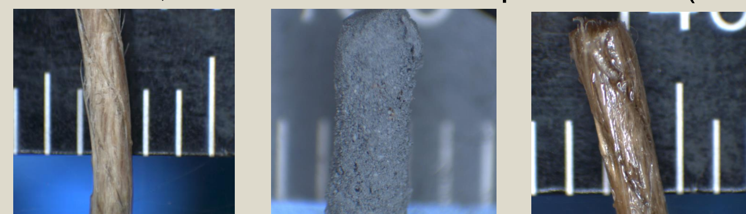
Figure 1: From left: uncoated twine, MCS-coated twine, and epoxy-coated twine. Scale in mm. (Agustines, 2022)
