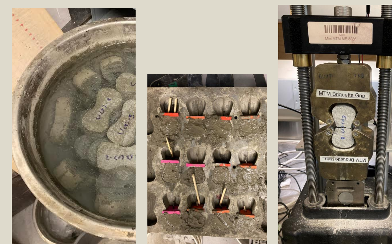
Figure 2: From left: curing dog bone samples, half dog bone samples, and the tensile testing setup (Agustines, 2022).
