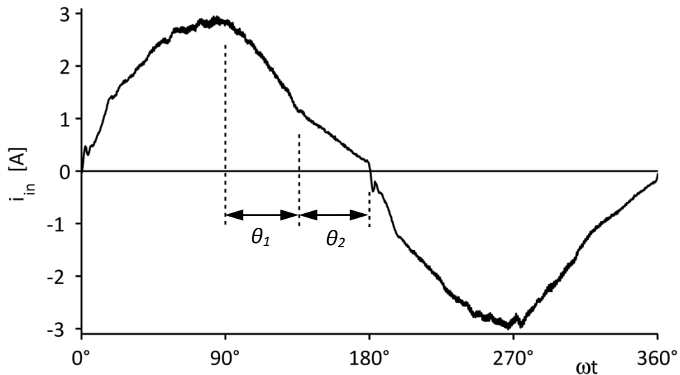
Figure 6.5: Measured input current waveform at rated load ( P_o = 202 \text{ W} ) with inductor 1 when the computed current is used for the current control; L^{imp} = 11 \text{ mH} , R_L^{imp} = 0.6 \Omega
