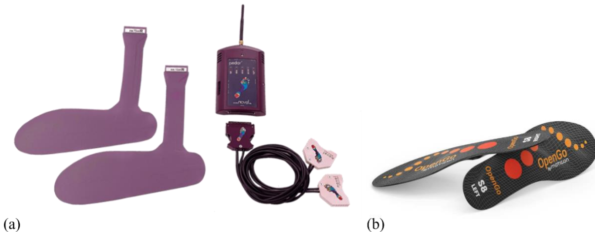
Figure 1-1 Research grade plantar pressure measurement systems (a) The Pedar™ system by Novel®, is a ‘gold-standard’ research grade plantar pressure measurement system with 99 sensors in a matrix configuration, (b) OpenGo™ by Moticon® a fully integrated in-shoe plantar pressure measurement system with 16 discrete sensors.
