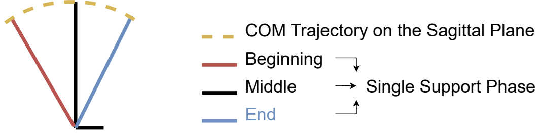
Figure 4.3: COM movements on the sagittal plane during the single support phase based on the inverted pendulum analogy. The black horizontal line represents the ball of the foot, while the long vertical lines in red, black, and blue indicate the beginning, middle, and end of the leg during the single support phase. The yellow dotted line represents the COM trajectory, which moves up and down like an inverted pendulum as the leg rotates.
