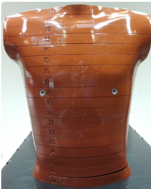
Figure 3.5: The Alderson Radiation Therapy anthropomorphic phantom.
