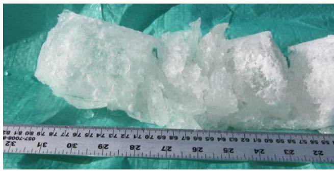
Figure 14. Horizontal profile of the second Athabasca ice core after it was removed from the ice auger.
