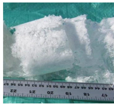
Figure 14. Horizontal profile of the second Athabasca ice core after it was removed from the ice auger.
