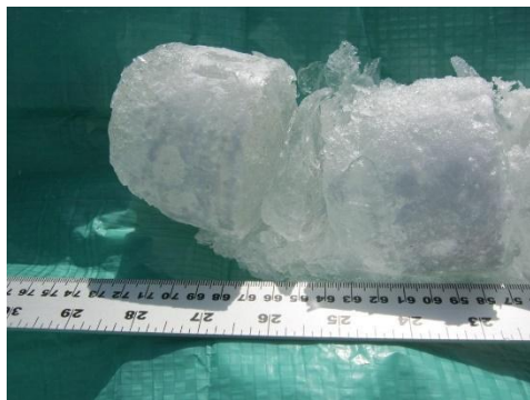
Figure 12. Horizontal profile of the Whitecourt ice core after it was removed from the ice auger.
