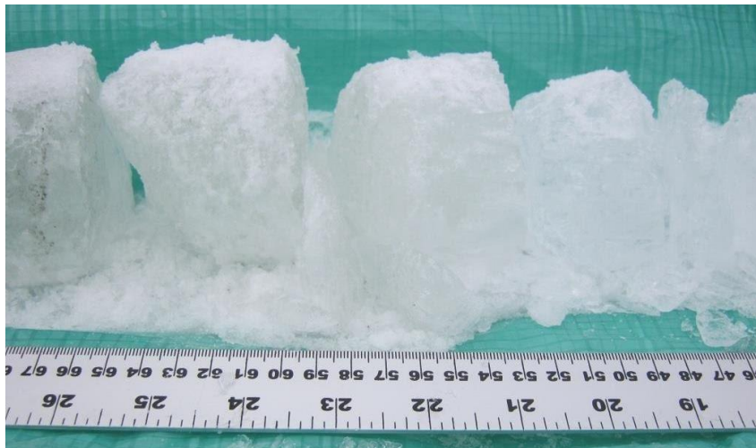
Figure 13. Horizontal profile of the first Athabasca ice core after it was removed from the ice auger.
