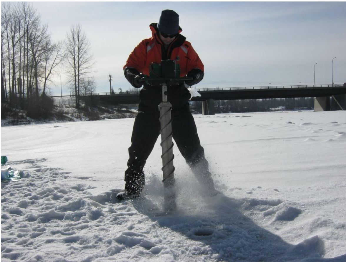
Figure 10. Ice cores were collected using an ice auger to drill into the ice.
