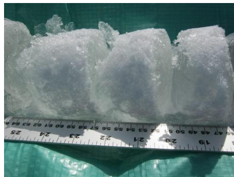
Figure 12. Horizontal profile of the Whitecourt ice core after it was removed from the ice auger.
