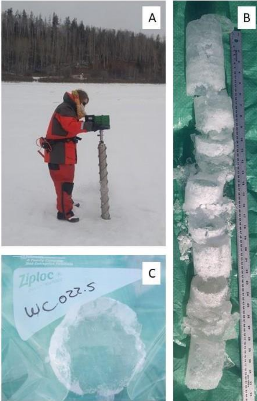
Figure 2.2: Steps in the collection of ice core samples. A) The use of an auger to collect an ice core, B) the ice core after it had been removed, beside a metre stick for reference, C) a section of ice core separated by either a natural break or manual cut.
