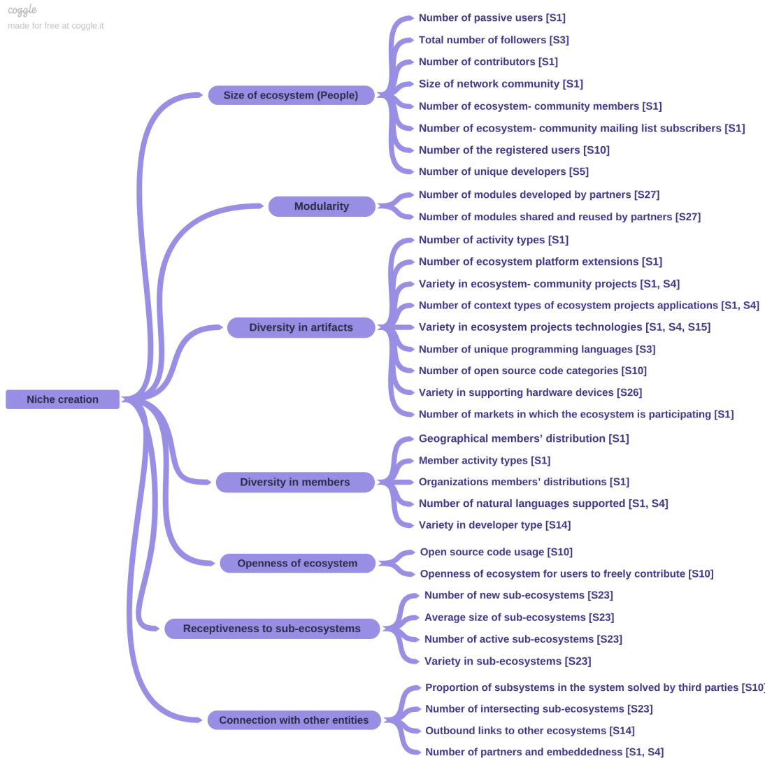
Figure 5.2: Sub-categories and metrics in the niche creation category within the software ecosystem health taxonomy
