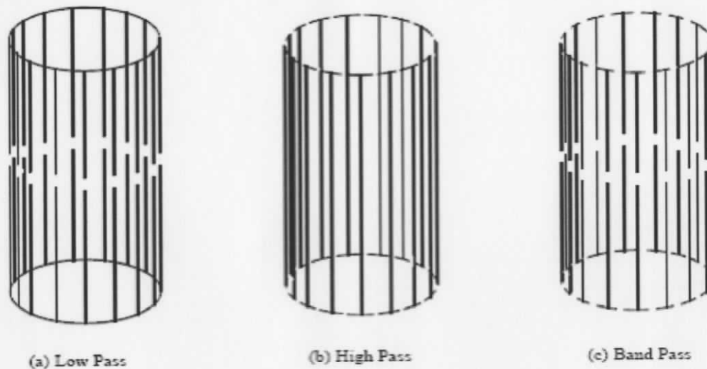
Figure 2-7: Configuration of the birdcage resonator
