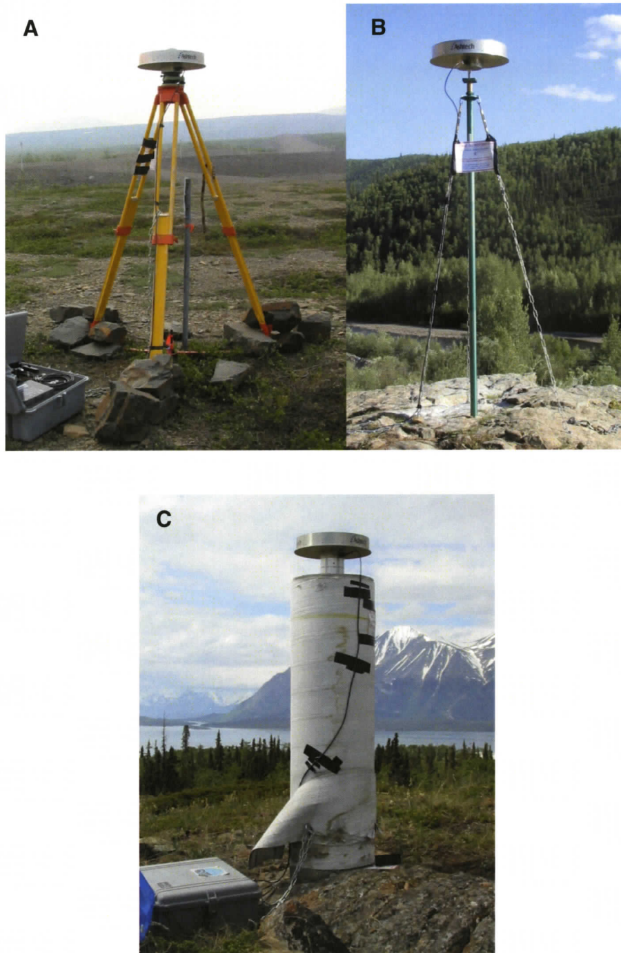
Figure 3.4. A. Example of a tripod set-up, at site RICH, Richardson Mountains, Northwest Territories. B. Example of a mast set-up, at site DAWS, Dawson City, Yukon Territory. C. CBN monument at site ATLI, Atlin, British Columbia.
