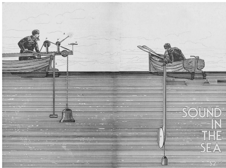
Figure 1.1: Illustration of Daniel Colladon’s experiments to determine speed of sound in water. [2]
