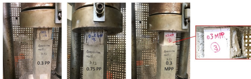
Figure 13. Fracture response of PFRCC specimens under compressive loading conditions.
