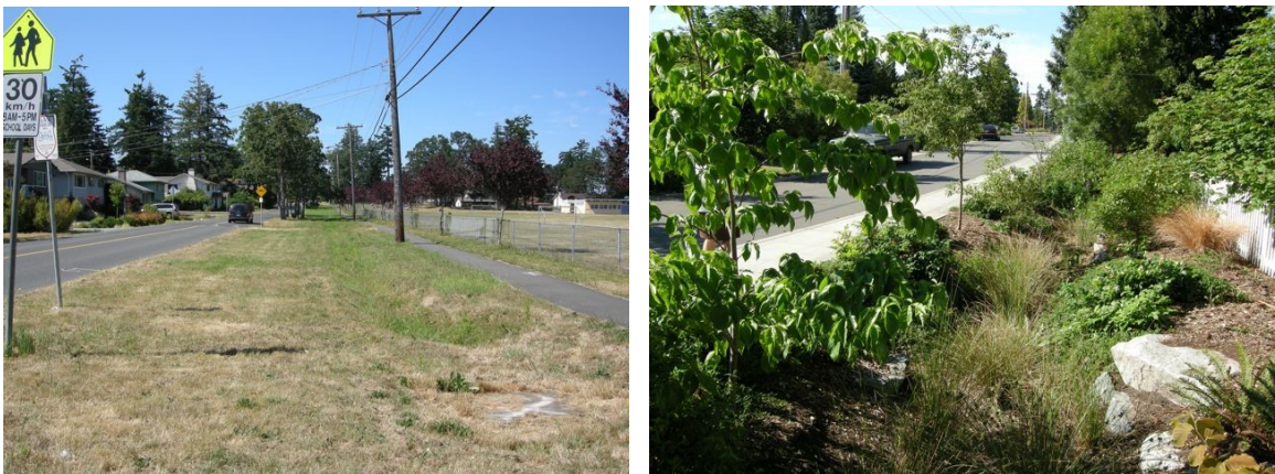
Figure 6.12. Example of a typical residential street boulevard in Swan Lake watershed (left), as it might look retrofitted with rain-gardens (Seattle SEA Street; right)
