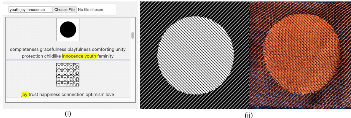
Figure 4.1: Textere's Pattern Library: (i) text tags matching users' text input are highlighted, (ii) weave draft designed, and final product woven
