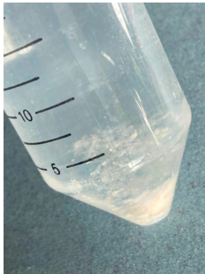
FIGURE 8 Crystals forming in Goodenough-kaolinite sample an hour after EtOH addition.
