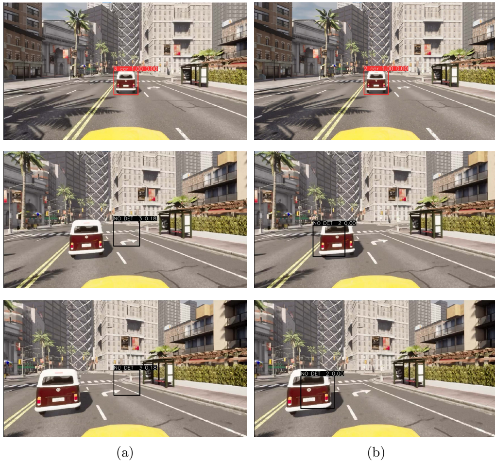
Figure 5.8: In this scenario, the object detection is missed, leading to failure in predicting the location of the object during lane-changing for Vanilla ByteTrack (a). ByteTrack + EMAP (b) significantly improves the prediction, successfully tracking the object in the next two frames.
