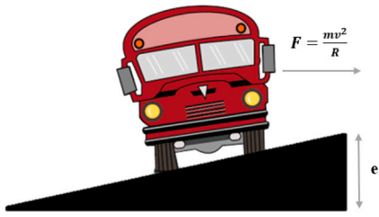
Fig. 2. Centrifugal force and highway superelevation.
