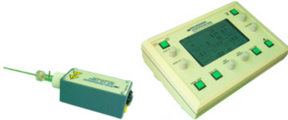
Figure 4.3: Axon Axopora 800A™ single-cell electroporator: headstage and micropipette assembly (left), and the digital console display (right).
