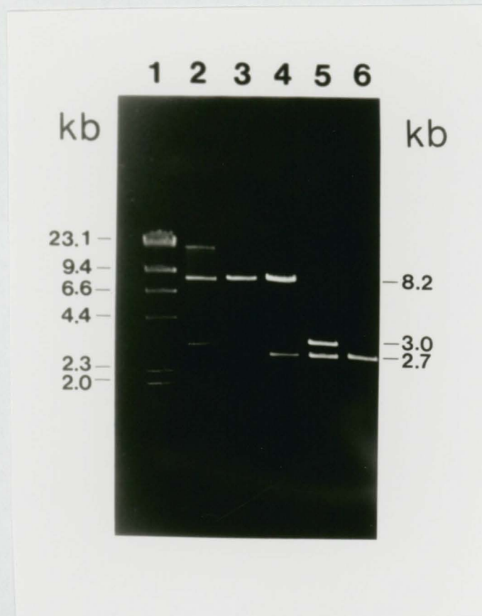
Figure 12 Electrophoretic analysis of the recombinant plasmids obtained from subcloning the 8.2 kb and 3.0 kb Bam HI fragments from pUV20 into pUC19.
