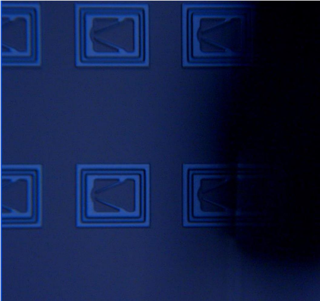
Figure 19: The micro-part is lowered to the plane of the double compliant beam slot
