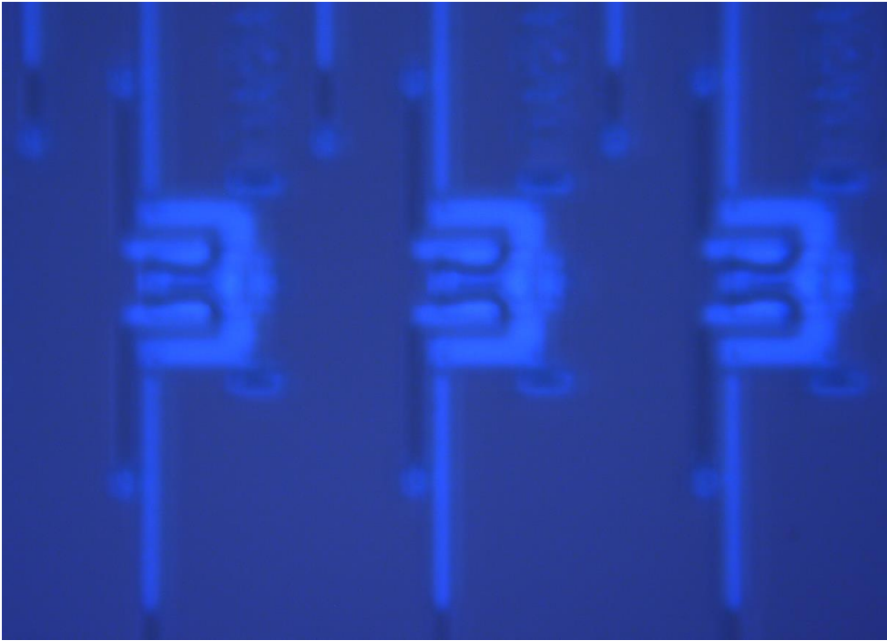
Figure 44: Three Micro-parts identified are in focus and have an average score of 940 with a minimum score requirement of 800
