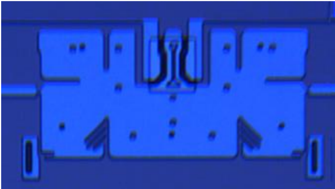
Figure 28: L-Edit design of the wide micro-part that utilizes the narrow micro-gripper
