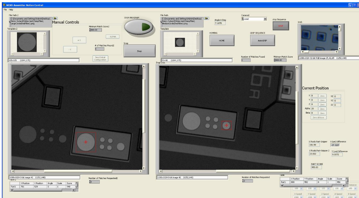
Figure 57: Unaligned geometry detected by computer vision
