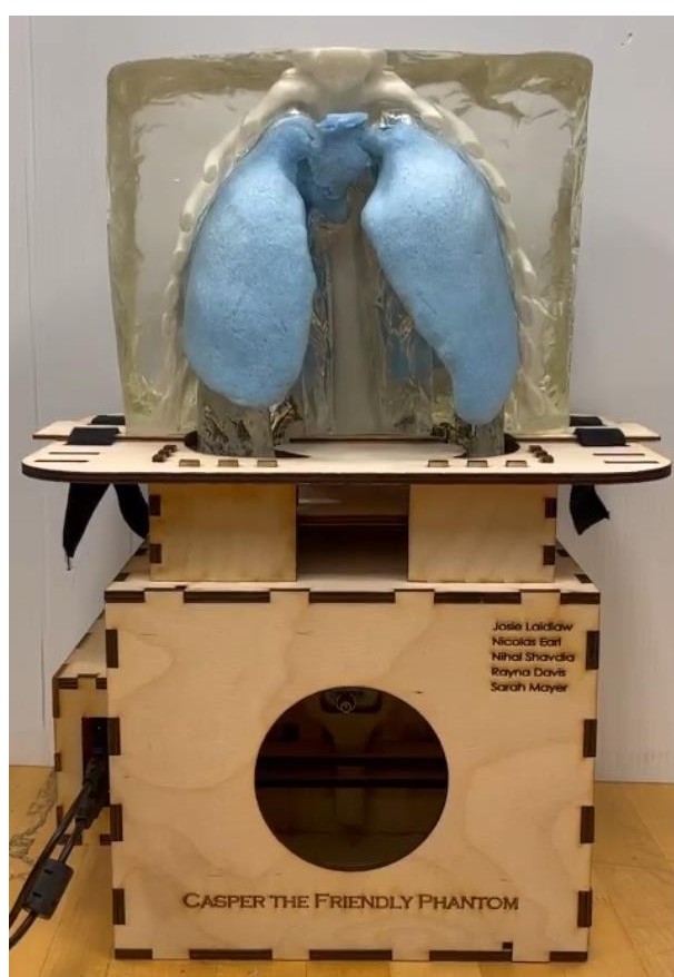
Figure 1. The fully assembled breathing phantom (CASPER) with one side of torso removed. This phantom is used to tune algorithms to account for lung movements.
