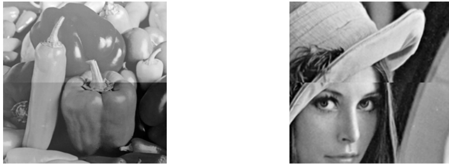
(a) Visible seam generated by photometric inconsistency between the input images (b) Discontinuous contours generated by previous registration errors
