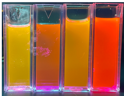
Figure 6 Rhodamine. B in chloroform, de-ionized water, ethanol and glycerol exposed to 365 nm UV light
