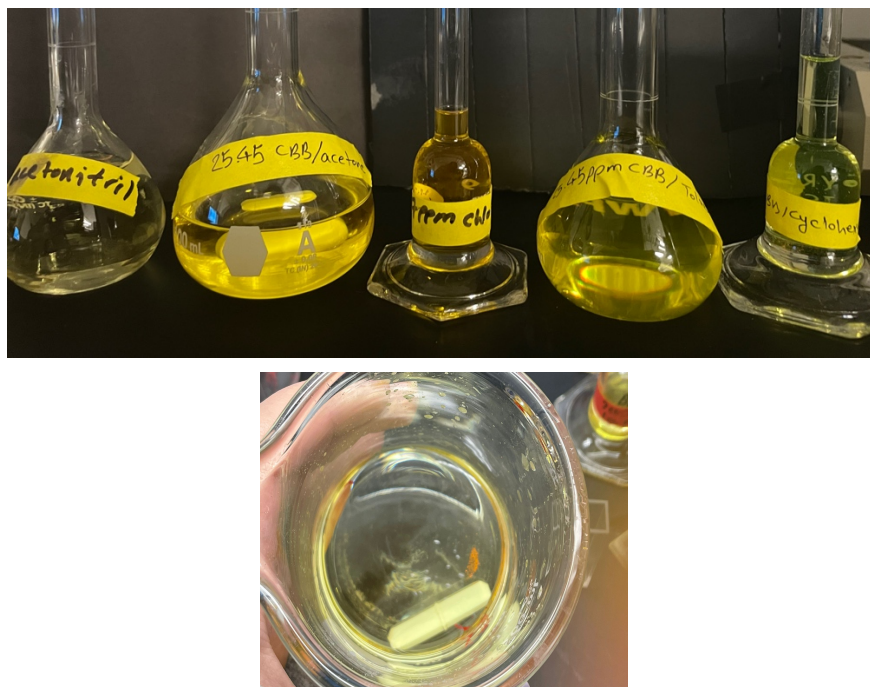
Figure 12 (top) Freshly prepared solution of CBB dissolved in acetonitrile – acetone – chloroform – toluene – cyclohexane from left to right (below) Peg400
