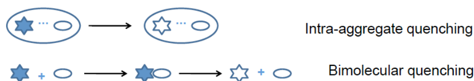
Scheme 3.1 Intra-aggregates quenching and bimolecular quenching (Shaded stars: excited chromophores, open ellipse: quenchers, and open stars: unexcited chromophores).
