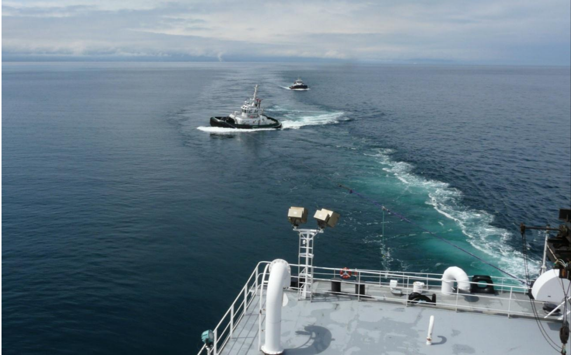
Figure 1.4: Escort Tug Foss America Escorting in Indirect Mode [Robert Allan Ltd.]
