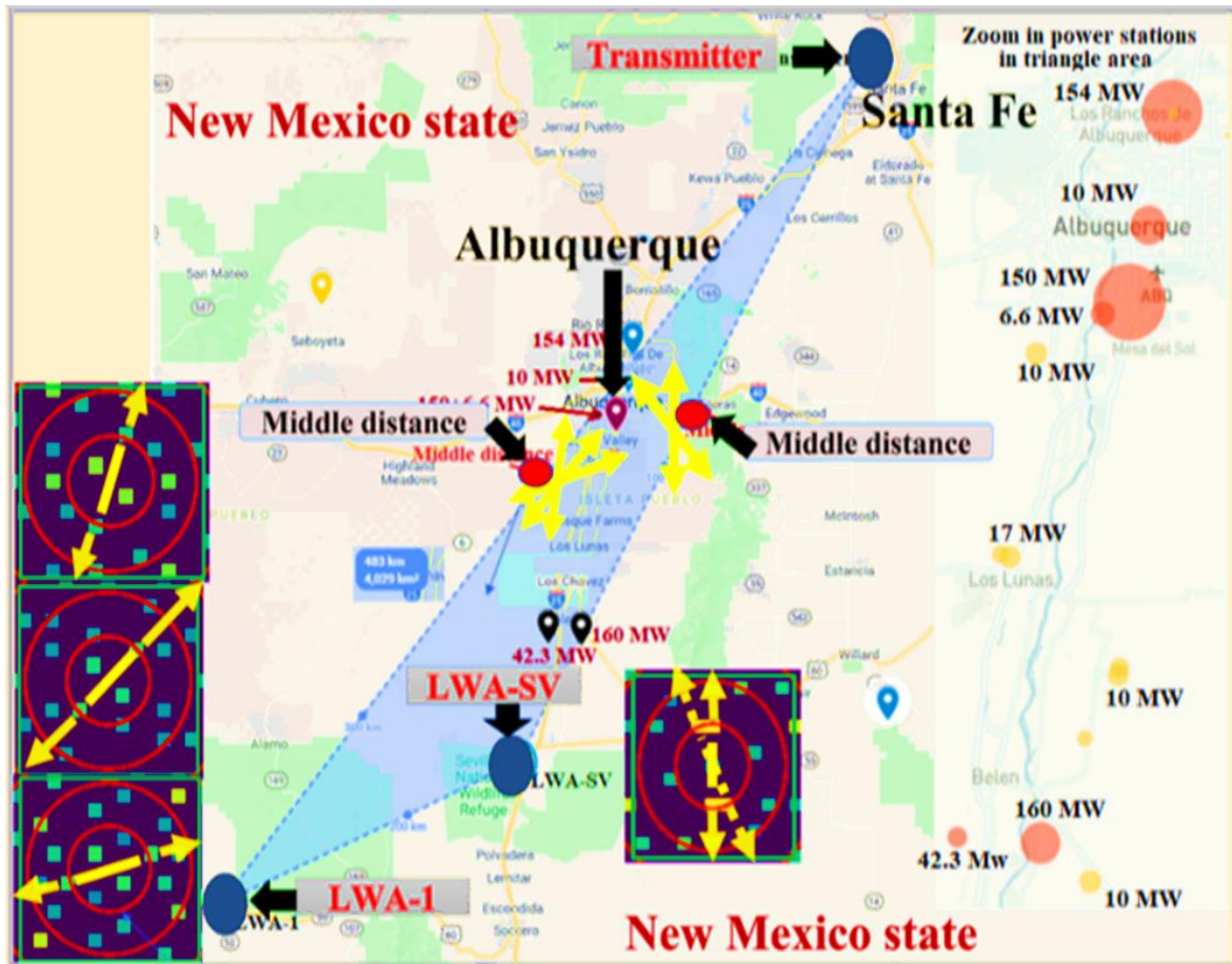
Figure 4.15 Measured wavevectors at mid-way points (red dots) between Santa Fe and LWA-1 and LWA-SV showing their intersections around Albuquerque and local power generating stations.
