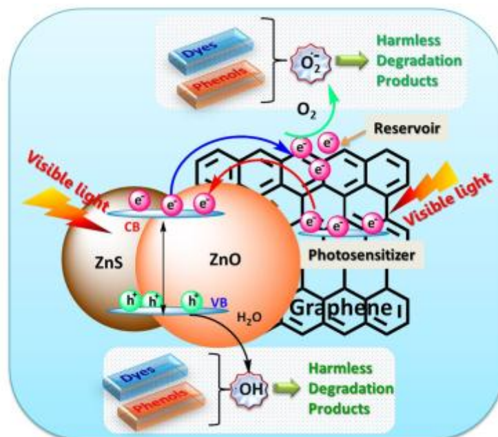
Figure 4.2 Schematic illustration of the charge separation and the transfer of photo-induced charge carriers in ZnS-ZnO/graphene heterostructured nano-photocatalysts for dye degradation under visible light irradiation [82]
