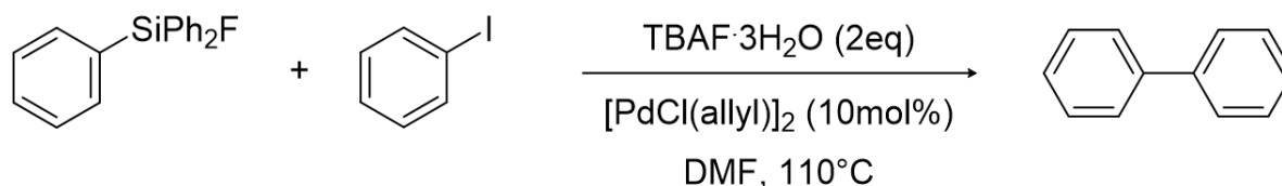
Scheme 3 Hiyama Cross-Coupling reaction of aryl iodides with fluorotriphenylsilane in the presence of 2 equivalents of TBAF and an allylpalladium chloride dimer catalyst.
