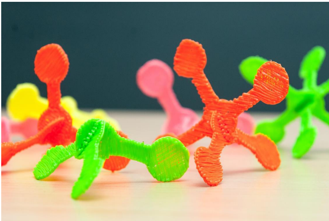
Figure 4.4 Sample of the molecular models produced using handheld 3D printing pens
