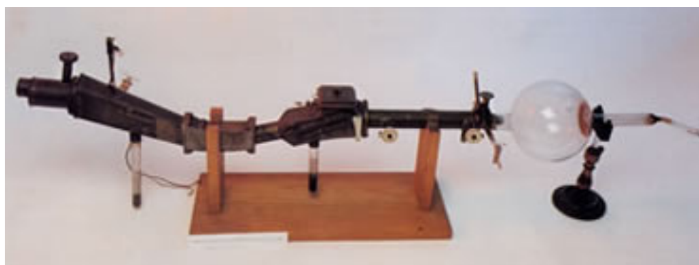
Figure 1.1. Image of Aston's third mass spectrograph displayed in Cavendish Laboratory museum. 7
