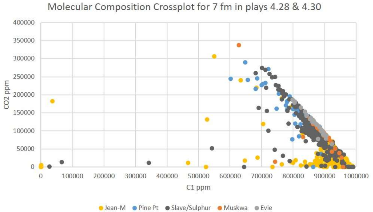
Figure B 104. MC map data – plays 4.28/30 MC (ppm) carbon dioxide methane plot for Jean Marie, Muskwa, Slave Point, Evie, Pine Point, formations [not to template].
