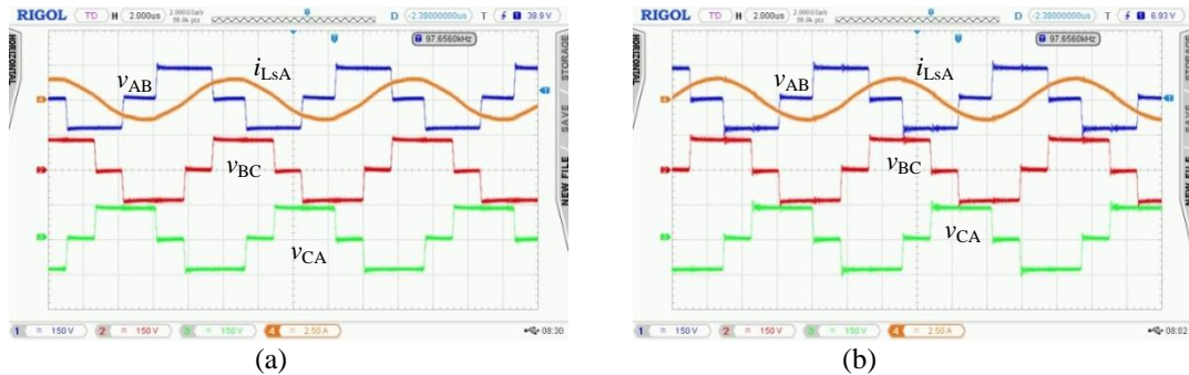
Fig. 4.65 Experimental waveforms of the voltage across the inverter terminals ( v_{AB} , v_{BC} , v_{CA} ) and the current through phase A of the tank circuit ( i_{LsA} ) of : (a) Module-1 and, (b) Module-2 for Case-5 : V_{in(min)} = 50 V, 20% of full-load, R_L = 300 \Omega , \delta = 102^\circ . Ch.1(Blue) - v_{AB} (150 V/div.), Ch.2(Red) - v_{BC} (150 V/div.), Ch.3(Green) - v_{CA} (150 V/div.), Ch.4(Orange) - i_{LsA} (2.5 A/div.). Time scale: 2 \mu s/div.
