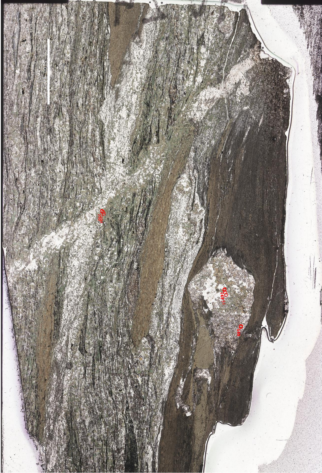
Figure B.9 AG137 Actinolite schist for EPMA. Large xenolith (?) on right.
