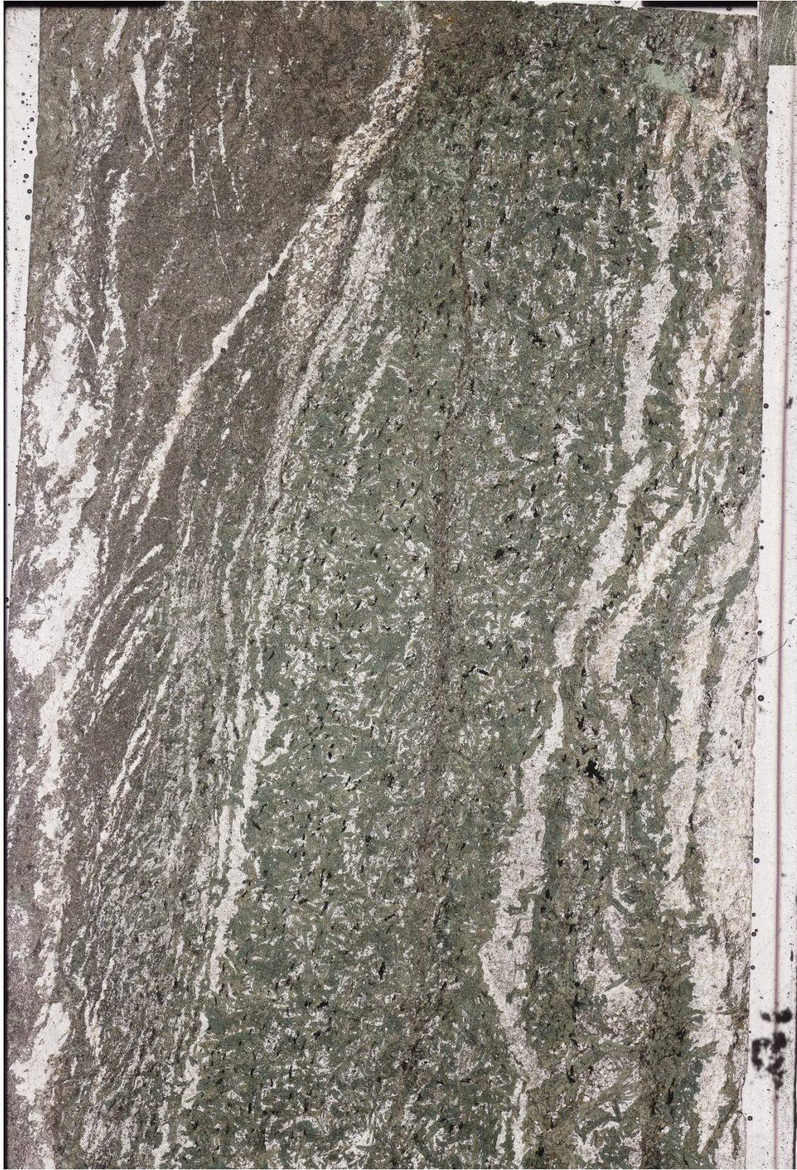
Figure B.19 AG119 thin section. Amphibolite with large ilmenite laths, from boudin in paragneiss.
