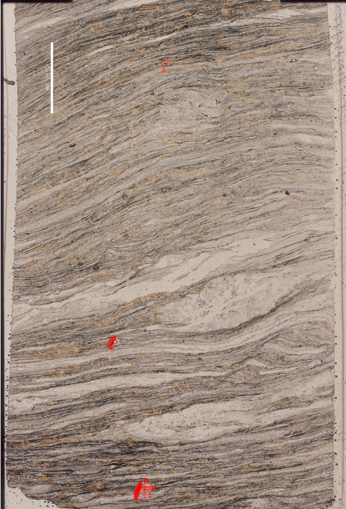
Figure B.10 AG067 thin section for EPMA gt-bt and RSCM.
