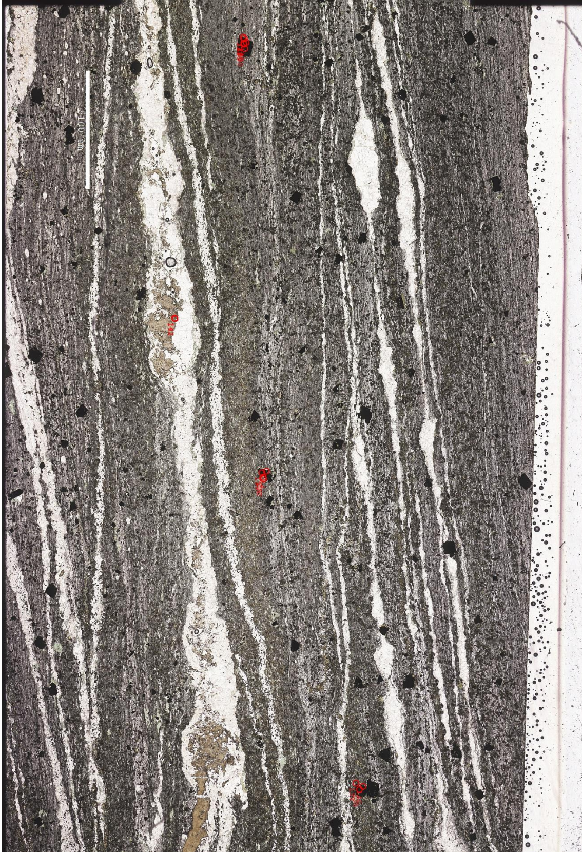
Figure B.8 AG055-1 thin section for EPMA with p/blastc magnetite in chl+ep mx.
