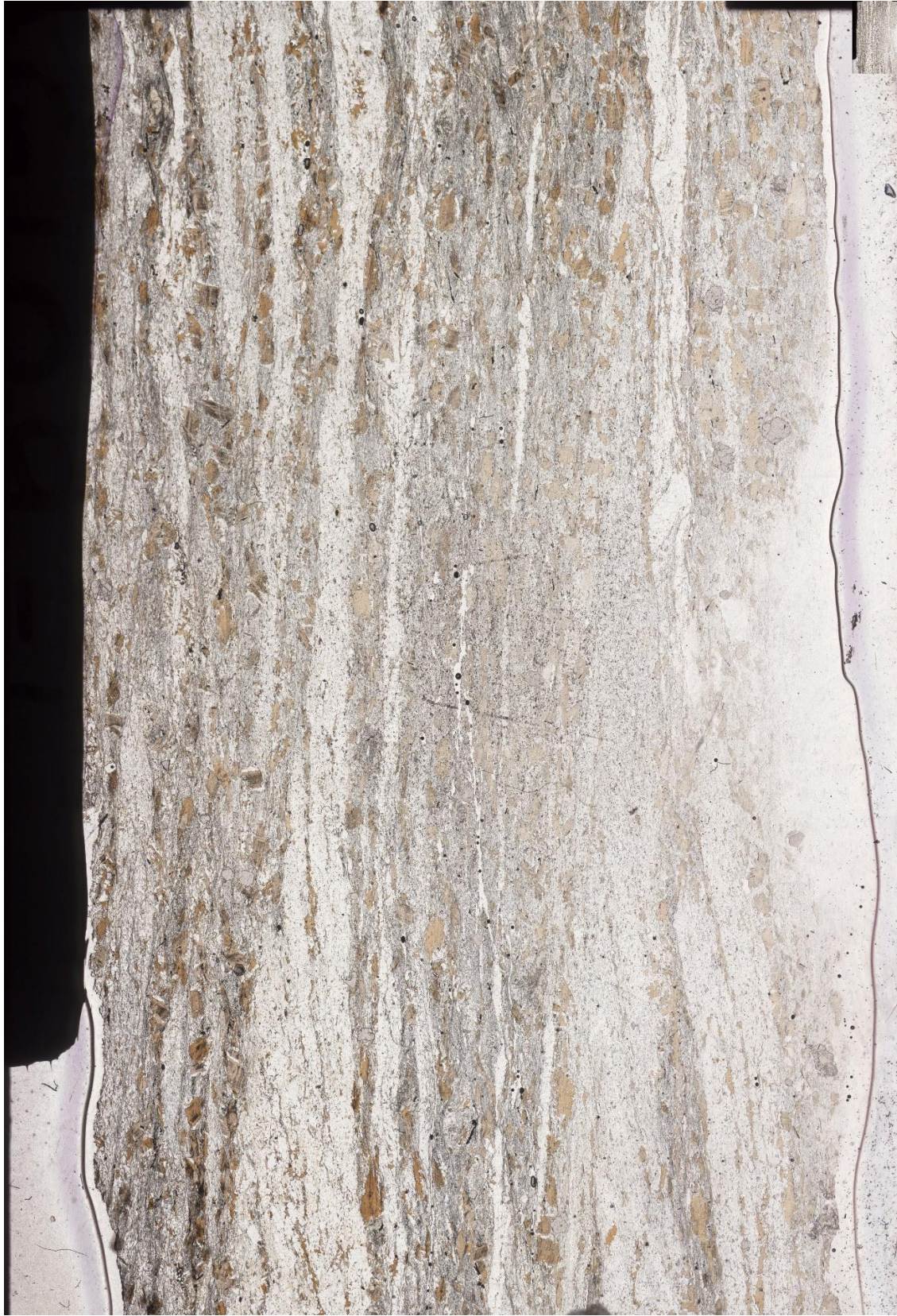
Figure B.21 AG109 thin section (EPMA for sulfide inclusions) Sillimanite zone.
