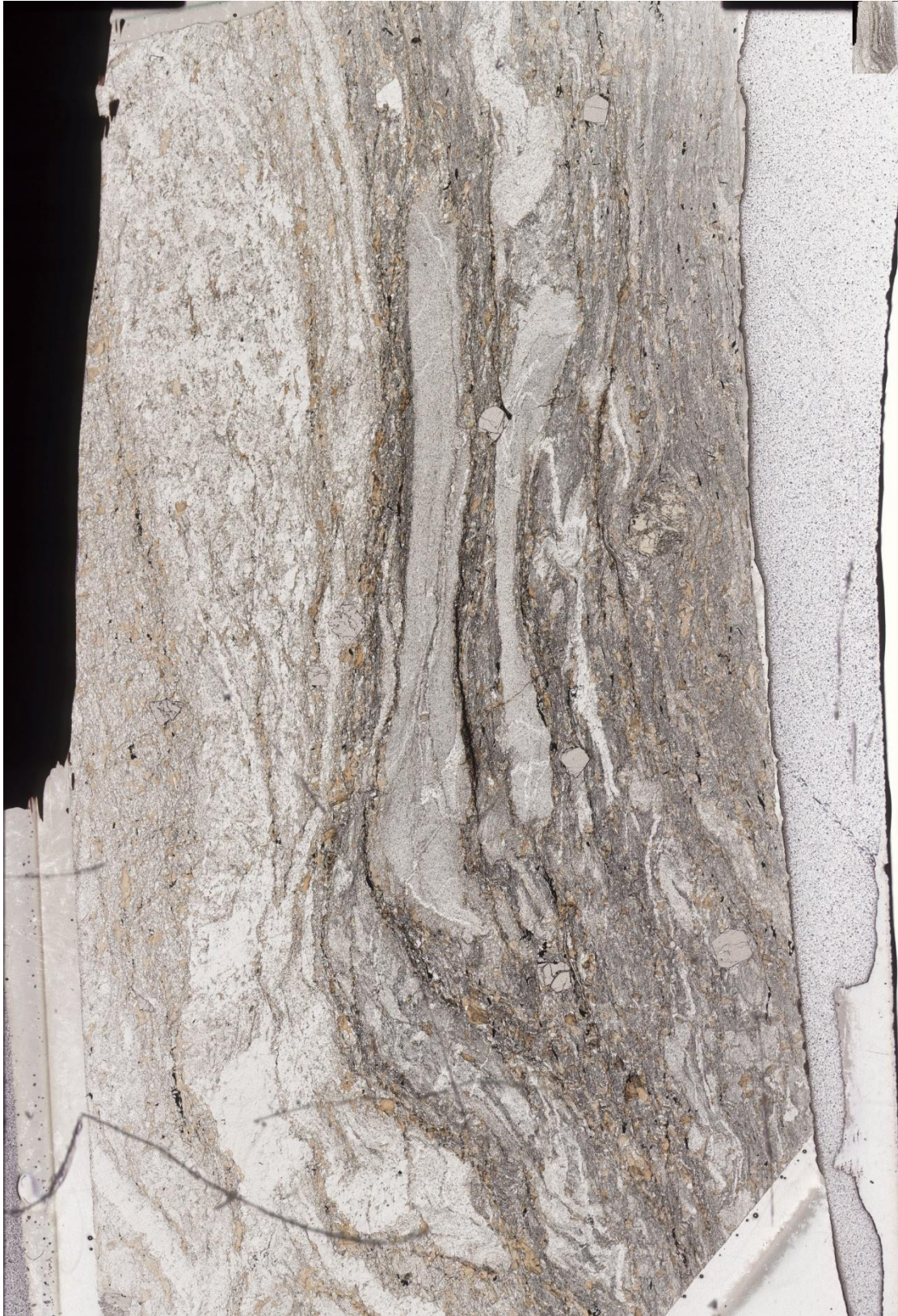
Figure B.12 AG011-2 thin section (unused for EPMA), showing compositional layering.
