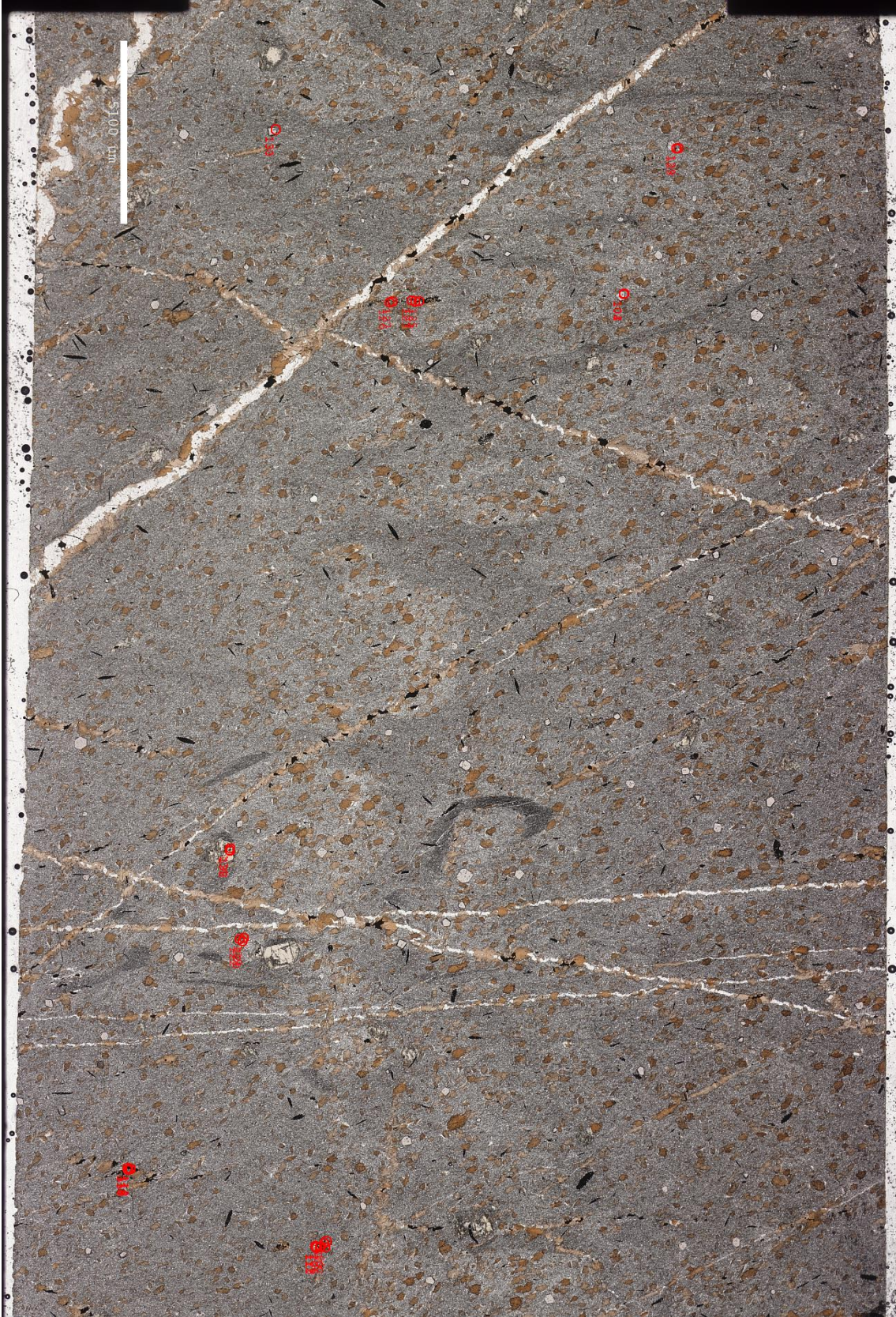
Figure B.22 AG049-1 for gt-bt and sulfide EPMA. Spotted gt-st-bt schist with coarse ilm.
