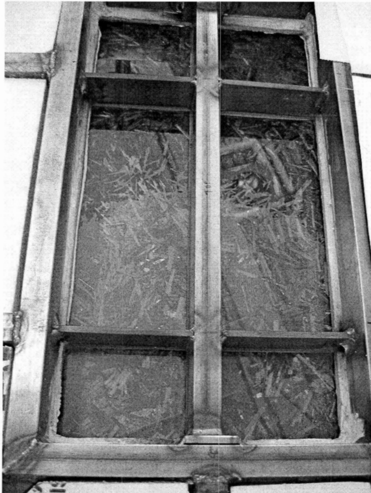
Figure 2.9: Resin Flow Pattern Through the Composite
