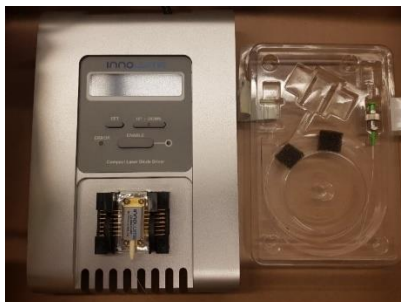
Figure 3.16 (Left) Top panel view of cLDD, showing LCD display, two status LEDs, control buttons, and 14-butterfly mount. (Right), Single mode optical fiber with an FC/APC connector.
