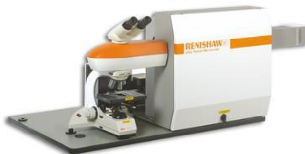
Figure 3.19 Renishaw Confocal Raman microscope
