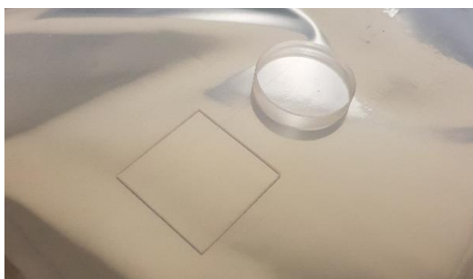
Figure 3.11 Slide vs disk vs window 170 \mu\text{m} thick.
