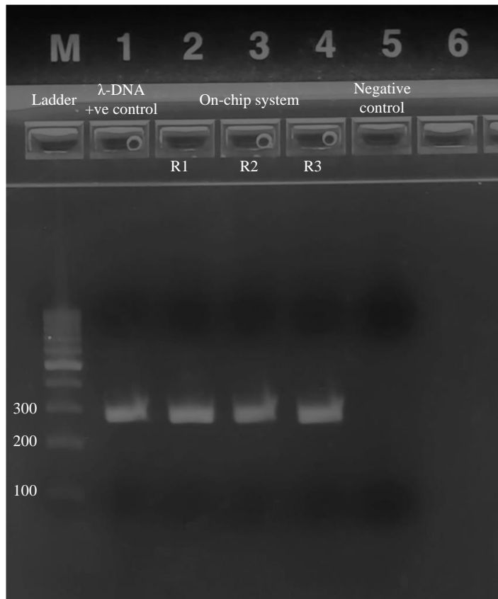
Figure 41 – E-gel results of the lab-on-a-chip device
